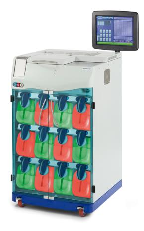
User friendly graphics and Intuitive HMI (Human Machine Interface) 2 Ports for easy and Innin Januarin automatic Reagent Remote Fill & Drain 1 Port for External Wax Dumping USB Port for Data Backup and Software **Automatic Upgrades** Sample Processing Chamber: · Entirely made of high quality Stainless Steel Special, easy to clean, surface treatment Gas piston to keep the lid open
